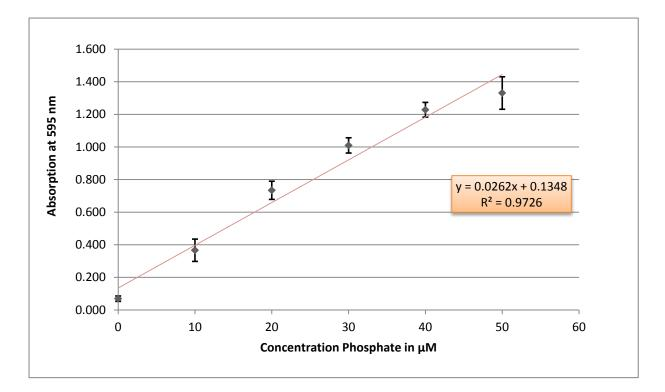
What we can see is that the more phosphate in the solution, the higher the absorption rate is. This is so because the phosphate absorbs light. The slope is practically constant. The last measurement is below the slope so it is possible that after a certain phosphate concentration the absorption stay constant.
