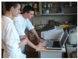
Picture 2: Measuring with the photospectrometer
