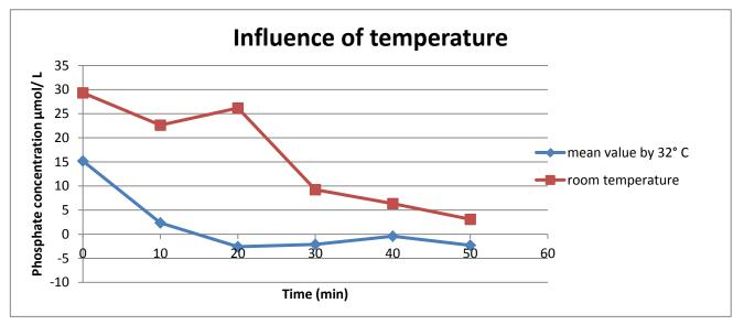
Figure 5 The influence of higher temperature in the phosphate uptake of yeast cells
