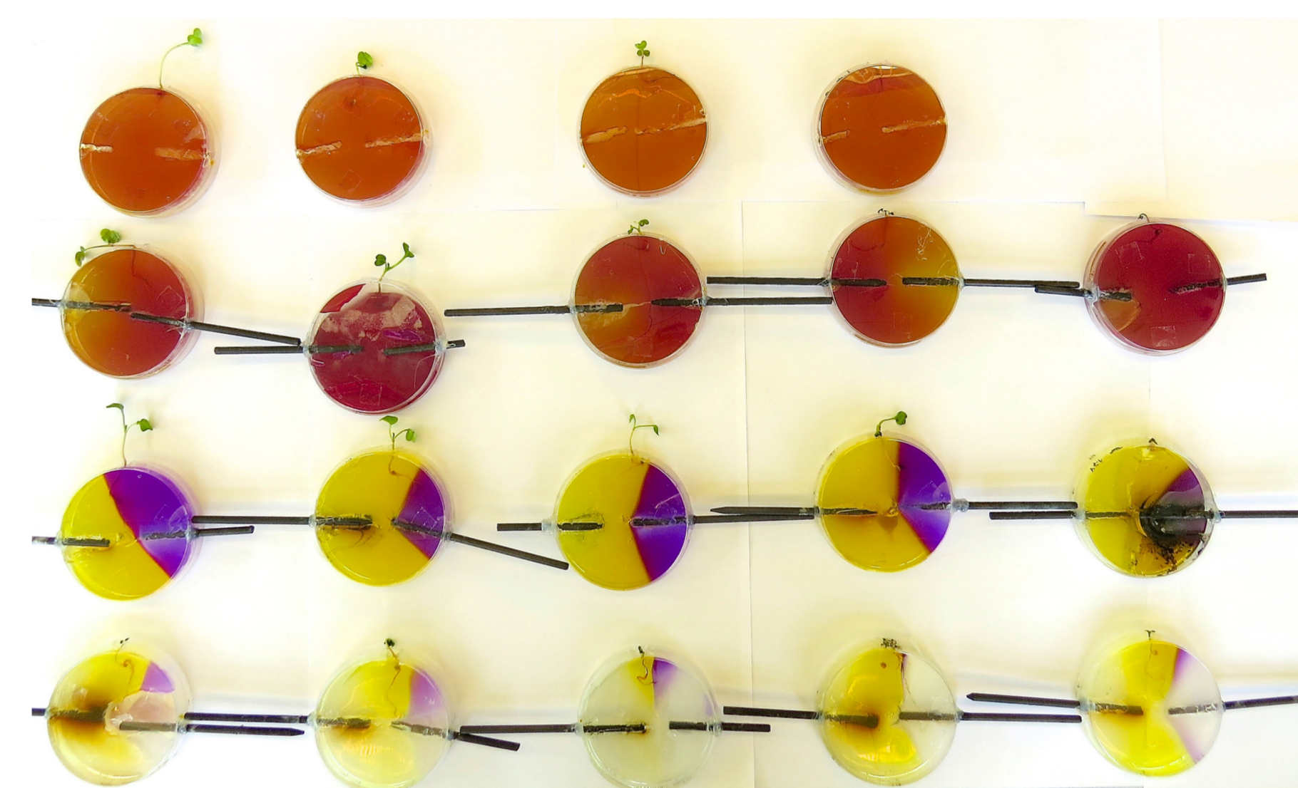
Figure 5: survey of the PH values (first line 0V, second 0.5V, third 1.5V, fourth 2.5V)
